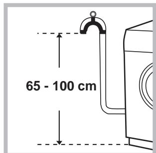
Connect the drain hose, without bending it, to a drain duct or a wall drain situated between 65 and 100 cm from the floor;
