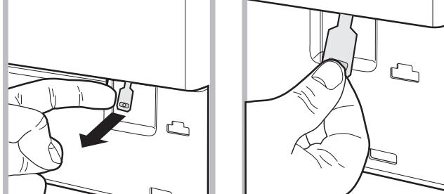
4. pull outwards using the tab as indicated in the figure, until the plastic tie-rod is freed from its stop position; pull downwards and open the door at the same time.
